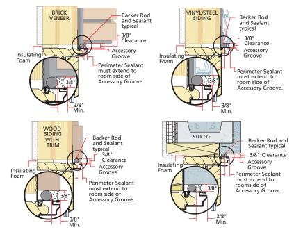
A. **Insert backer rod** into the space around the door so there is approximately 3/8" to 1/2" clearance between the backer rod and the exterior face of the door.
